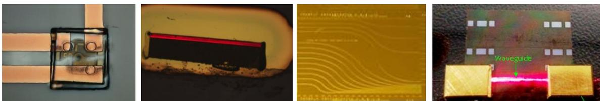
*Images of embedded and connected VCSEL; (red) light reflection from the imprinted mirror; an imprinted waveguide and fibre blocks connected to polymer waveguide with one channel lit by a red laser.*
