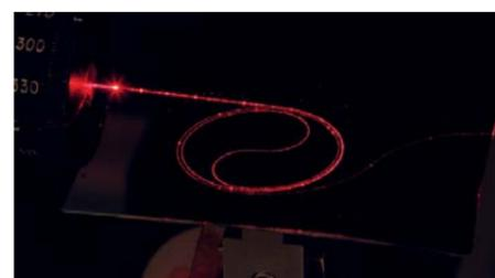
Red light travelling in a 27-cm long spiral waveguide (note: waveguide is designed for 1550 nm, thus it is not single-mode and optimal at 633 nm)
