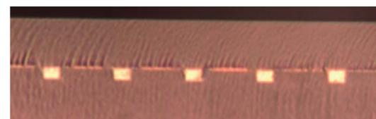
Cross-section of an array of five parallel optical waveguides. Waveguide width 6  $\mu\text{m}$  and height 4  $\mu\text{m}$
