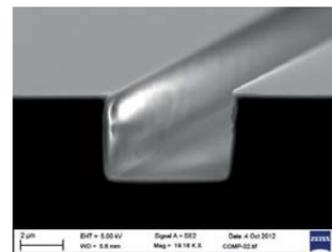
SEM picture of imprinted waveguide trench
