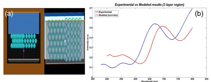
(a) Three layer modelled photonic crystal structure having mix of rectangular and hexagonal lattice. (b) Agreement between simulated and experimental results.
