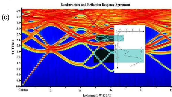
(a) Modelled FCC structure with waveguides (b) Reflection response from the structure (c) An agreement between bandstructure and reflection response.
