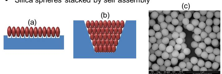
(a) Single layer of spheres placed on seed layer (b) Photonic crystal formed by self assembly of the spheres (c) SEM image of the sample formed by self assembly of silica spheres.
