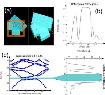
(a) Modelled core-shell structure with waveguides (b) Reflection response from the structure (c) An agreement between bandstructure and reflection response.
